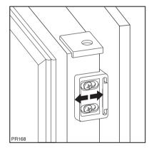
Fix cover (D) on guide (B) until it clips into place.
